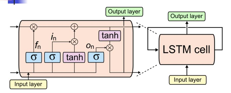
Repeating modules for the LSTM neural network: input layer, LSTM layer with one LSTM cell, and output layer.
